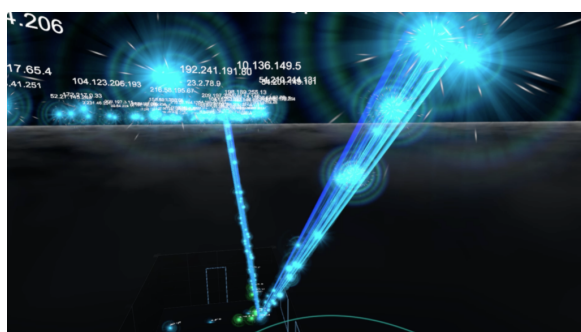
Figure 13: Netflix streaming traffic. A high-bandwidth stream like this can cause the visualization to fall behind real-time as it renders each packet in the stream.
