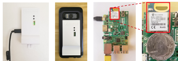
Figure 7: Decawave localization system. To localize mobile devices, we used the commercially available Decawave MDEK1001 kit, which provides decimeter accuracy at 10 Hz. Left to right are depictions of anchor, tag, gateway, and module. The UWB module is small and could be integrated into smaller tags. Four anchors covered a 15.5m x 4.5m room.
