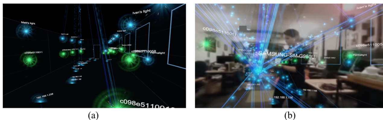
Figure 8: Local host placement. Local devices are placed in a digital twin of the room using location information provided by the system representation. Green orbs represent Thread devices, and blue orbs represent WiFi devices. If the physical location of a local device is unknown, then it is embedded randomly in the floor (a). Device locations are updated each time step, reflecting the latest localization information. In (b), as the smartphone moves, packets sent to it from the WiFi-enabled smart lights follow the phone’s location.
