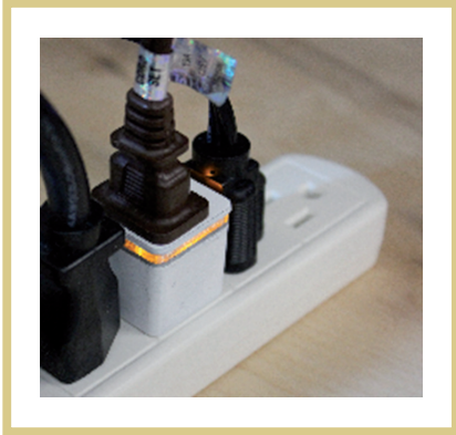
Figure 7. PowerCube, a cubic-inch plug-through power meter. Although this design achieved our volume target, it was difficult to assemble due to the use of six interlocking circuit boards that formed a cube.
